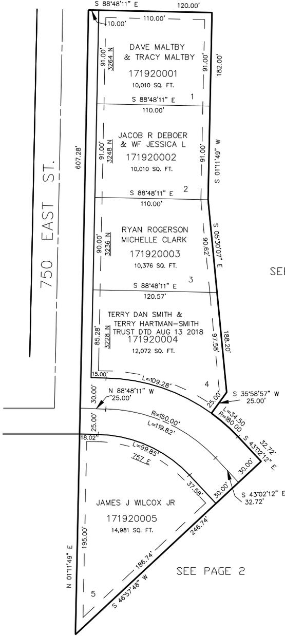
7' UTILITY & DRAINAGE EASEMENTS EACH SIDE OF PROPERTY LINES AS INDICATED BY DASHED LINES EXCEPT AS OTHERWISE SHOWN.
